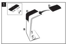
Cut the rubber tube (D) (5 cm each side) and fit the bracket (B).
