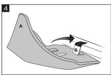
Put the skid plate (A) being sure that the bracket (B) is inserted in the frame.
