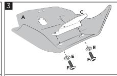
Fix the bracket (C) to the skid plate (A) using the screws (F) and washers (E).
